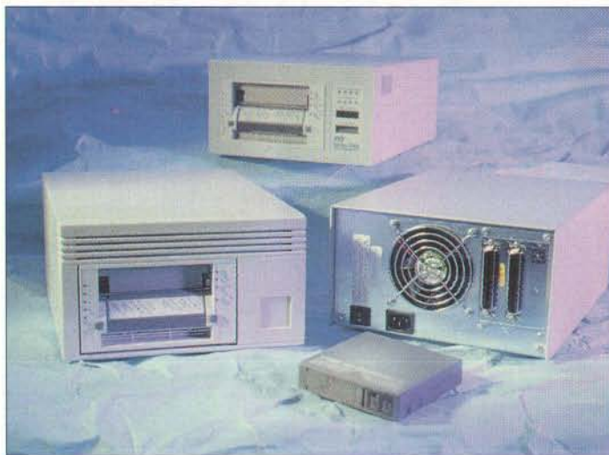
The outside cases of the three DLT drives we tested are virtually identical. All are manufactured by Quantum. Clockwise from the top: TTI's CTS-2110 drive showing its LED panel on the front (which the other drives don't offer), the back of Overland Data's DLT 2000 drive showing its SCSI ports and fan, and Quantum's DLT2000 drive.
