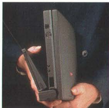
Small notebooks are becoming more capable thanks to better components and clever designs. DEC's HiNote Ultra features an optional floppy drive that docks to the underside of the portable. Other small notebooks like the HP OmniBook 600 and Gateway 2000 Liberty PC still use the older external floppy drive design, where the drive hangs off the side of the portable.
